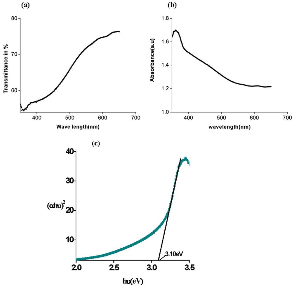
FIG. 2. (Color online) UV-vis spectrum of ZnO thin film: (a) Absorption spectra, (b) optical transmittance spectra, and (c)  $(\alpha h\nu)^2$  vs  $h\nu$  plot for estimation of band gap.
