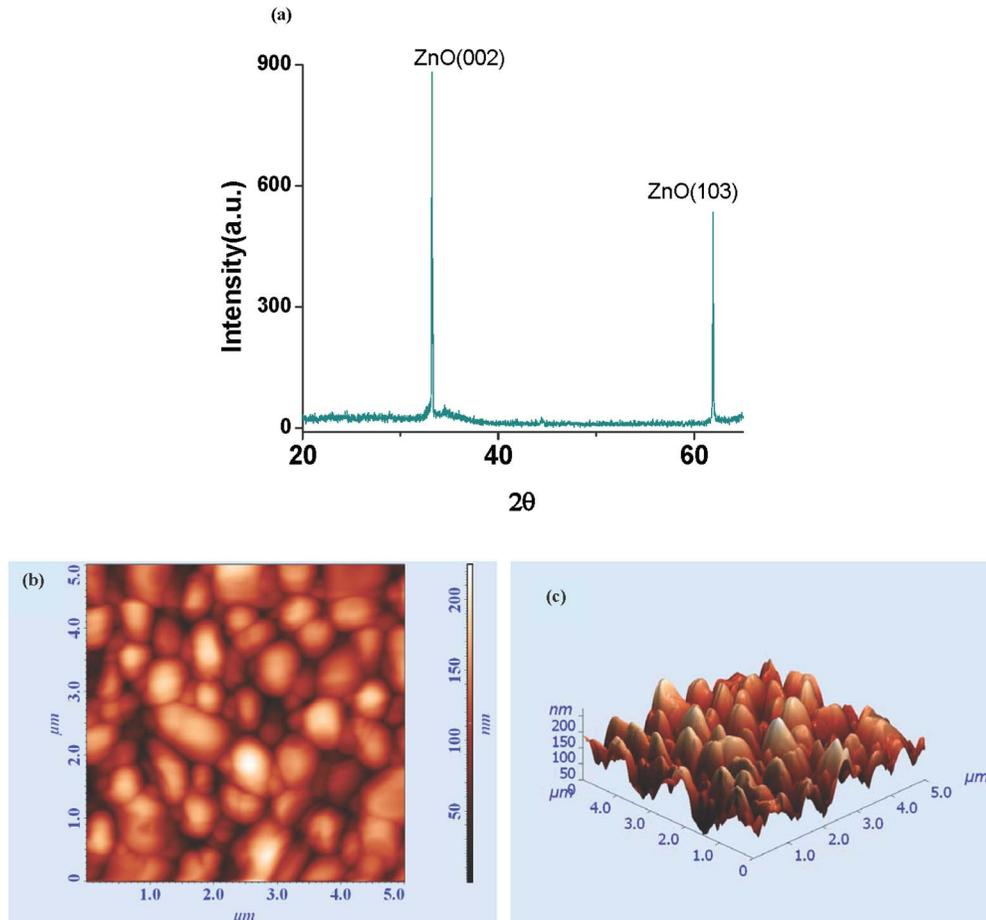
FIG. 1. (Color online) XRD and AFM images of ZnO film: (a) typical XRD pattern, (b) AFM 2D image, and (c) Corresponding 3D image of (b).
