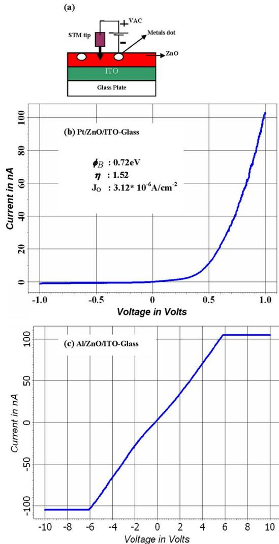
FIG. 3. (Color online)  $I$ - $V$  characterization: (a) Measurement setup, (b) rectifying characteristics of Pt contact, and (c) Ohmic  $I$ - $V$  plot of Al/ZnO contact.
