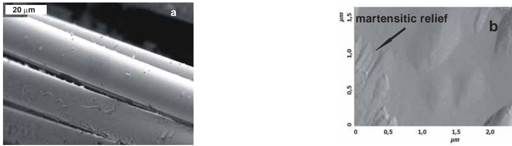
Fig. 5 a, b. The \text{ReZrO}_2 -coated Hi-Nicalon™ fiber after oxidation at 1000C: a – SEM image, b - AFM image.
