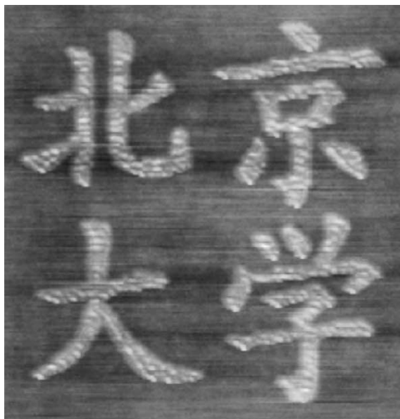
Fig. 4. AFM topographic image of a pattern of Chinese characters formed with a static voltage. Image size: 2\ \mu\text{m} \times 2\ \mu\text{m} .
